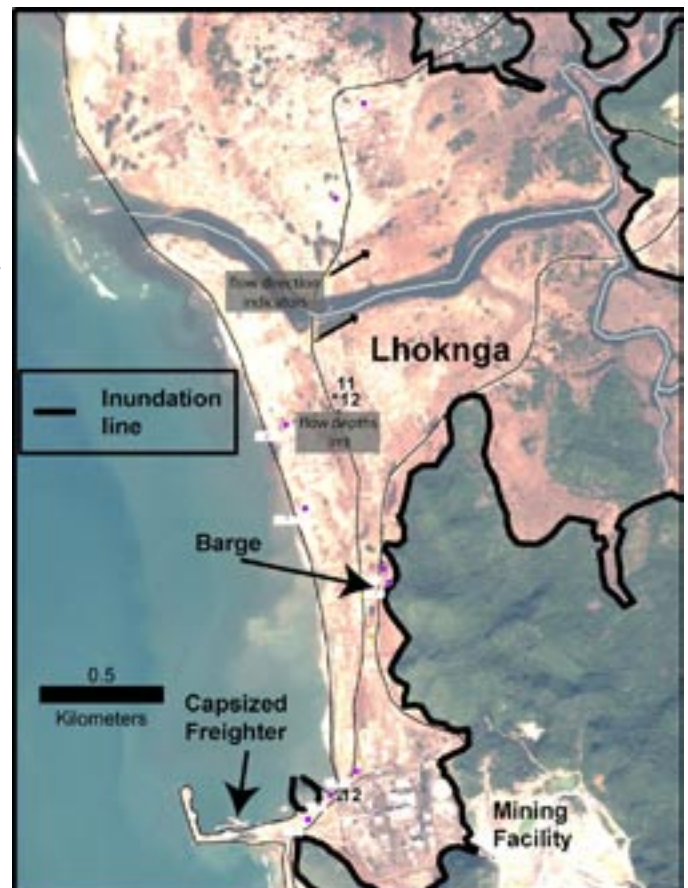
Figure 4. Satellite view of Lhoknga. The estimated runup at the trim line above the barge was 25 m.
