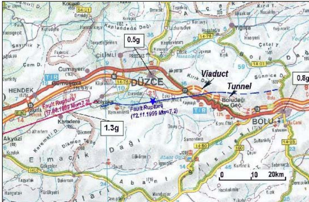
Figure 4 Peak horizontal ground accelerations recorded in the Düzce earthquake.
