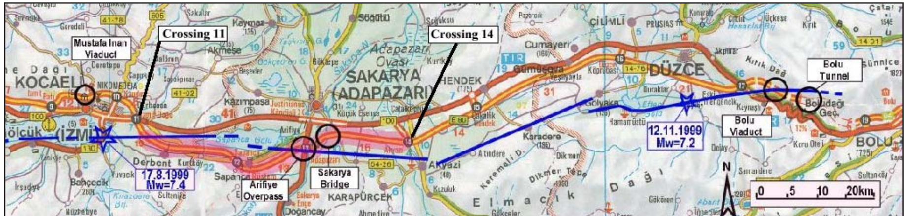
Figure 6 Location of highway and viaduct damage in the Kocaeli and Düzce earthquakes. The fault ruptures are indicated by blue lines, and the two stars on these lines show the epicenters of these earthquakes. Most of the highway damage occurred to the section between crossing 11 and crossing 14.
