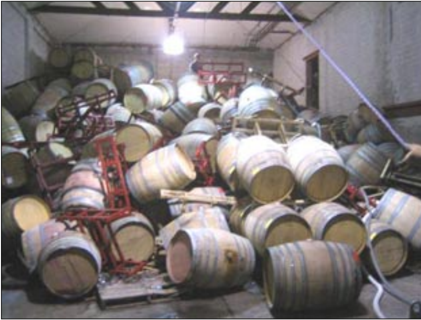
Figure 12. Collapsed wine barrel stacks at Turley Wine Cellars, SR 46 near Paso Robles (photo Marrow).
