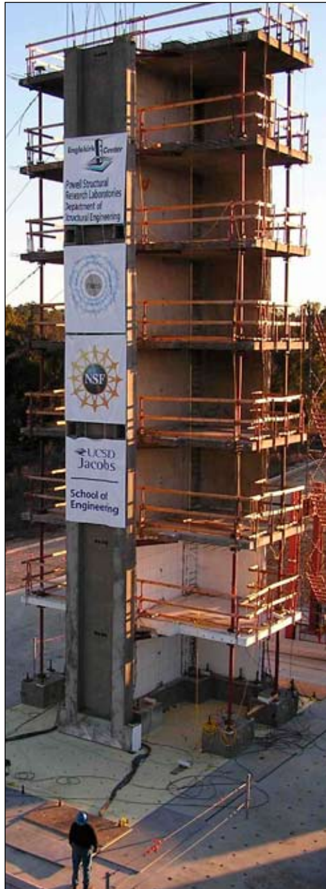
Full-scale, seven-story, reinforced concrete building on shake table.
