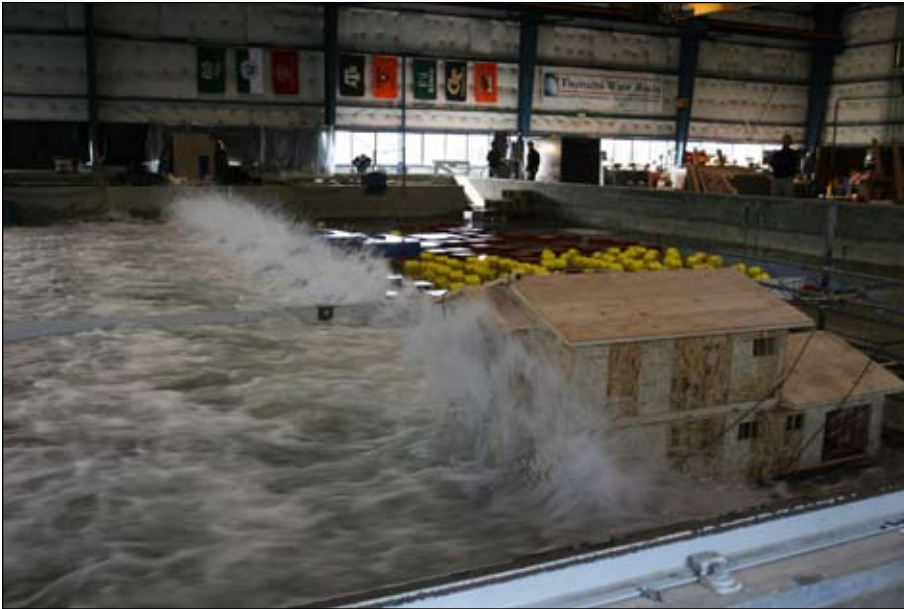
Waves impacting a 1/6-scale residential wood house at the NEES Tsunami Research Facility.
