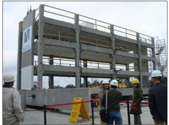
Million-pound concrete structure on UCSD shake table.
