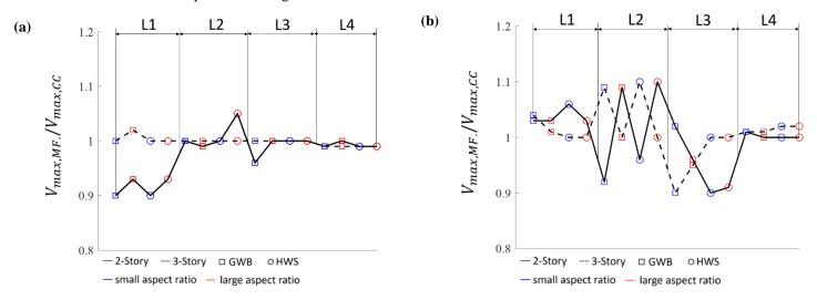
**Fig. 3** Ratio of maximum base shear from pushover response between OMF-retrofitted archetypes and SCC-retrofitted archetypes is presented for the X-direction (a) and Y-direction (b).
