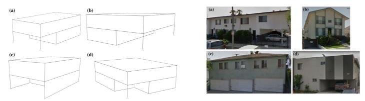
**Fig. 1** Schematic isometric views of typical SWOF woodframe building configurations (Burton et al. 2019) identified from survey (left), along with photos of typical SWOF woodframe building configurations (right): **a** L1, **b** L2, **c** L3 and **d** L4
