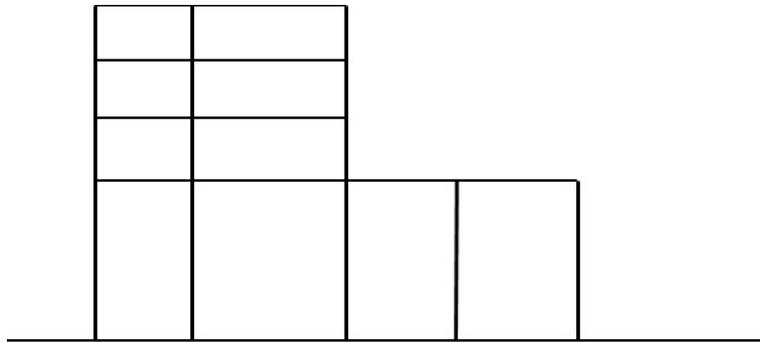
**Figure 4: Vertical Irregularity (building elevation view shown)**
