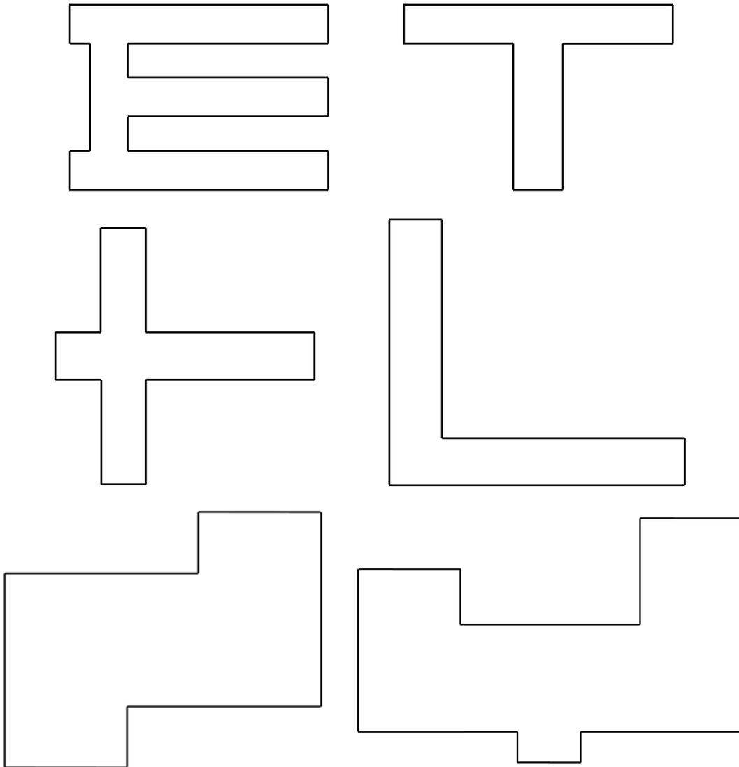
**Figure 5: Plan (Horizontal) irregularities showing re-entrant corners**
