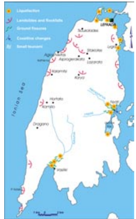
Figure 8. Geological and geotechnical effects of the Lefkada earthquake.
