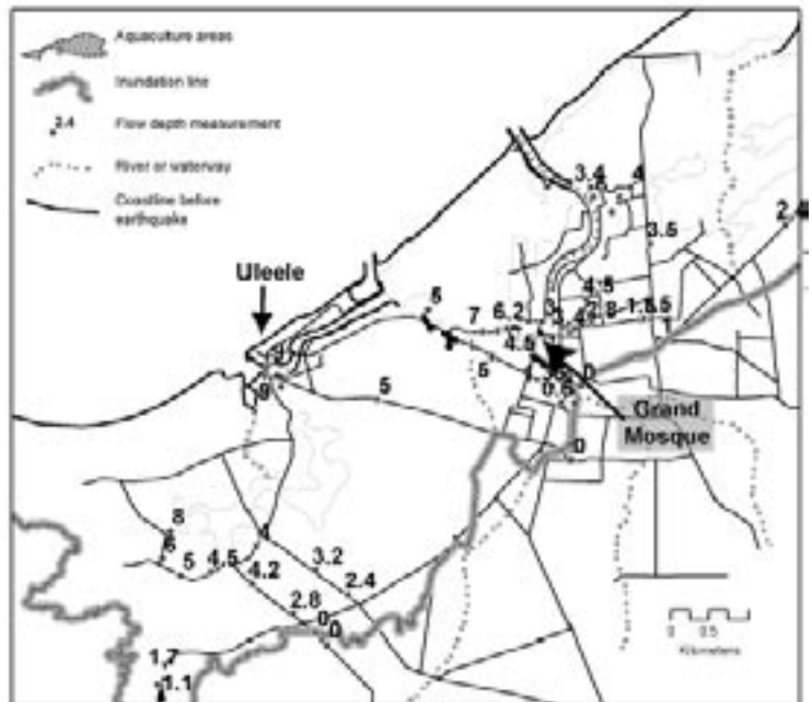
Figure 2. Map of Banda Aceh with flow depths as measured in the field.
