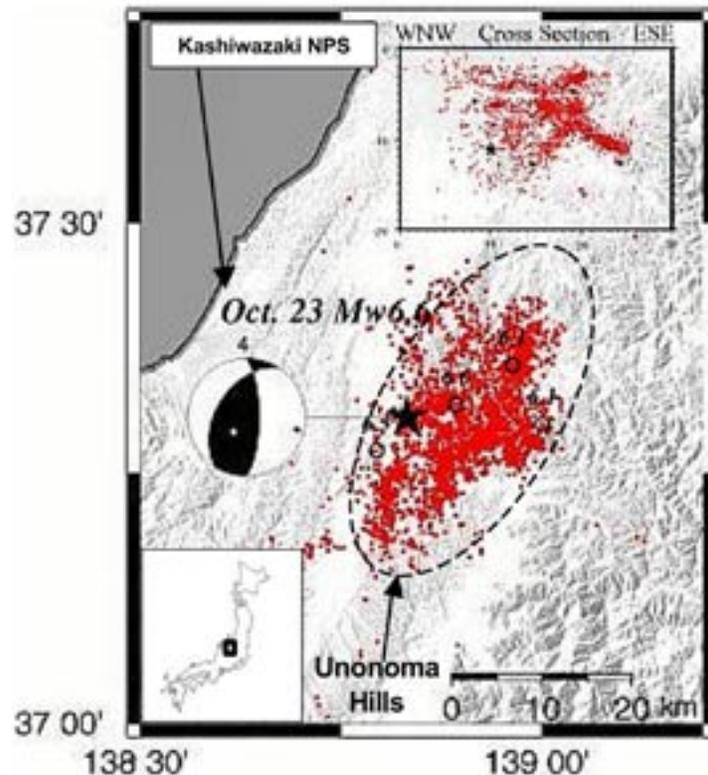
**Figure 1.** Aftershock pattern and mechanism. The Unonuma Hills are approximately outlined by dashed ellipse, and the Shinanogawa Lowland is the white area to the west (adapted from original figure by Group for Joint Observation, Kyoto and Kyushu Universities).
