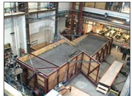
*Testing of HDPE pipe for fault offset.*
