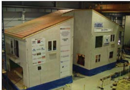
*The townhouse building spanning the two 3-D shake tables at the University at Buffalo NEES facility prior to undergoing the 3-D Northridge ground motion.*
