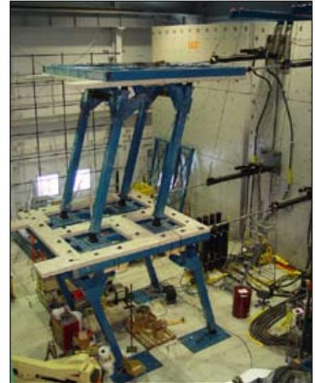
*The NCS features a two-story-high, four-column swivel test frame supporting two steel grid platforms that represent two adjacent floor levels. The system uses four hydraulic actuators that push and pull the platforms up to 40 inches in each direction, at velocities of 100 inches per second, simulating in real time how upper floors move during earthquakes.*
