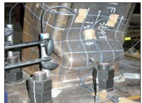
*Plastic hinging and severe local buckling occurred at the bottom and top of the first-story columns, with little evidence of significant girder yielding (photo: Maison/Kasai).*
