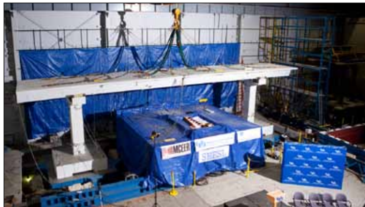
Half-scale bridge undergoing testing at SEESL.
