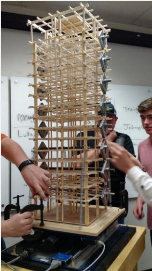
Figure 1: Students secure their structure to the shake table for seismic testing.
