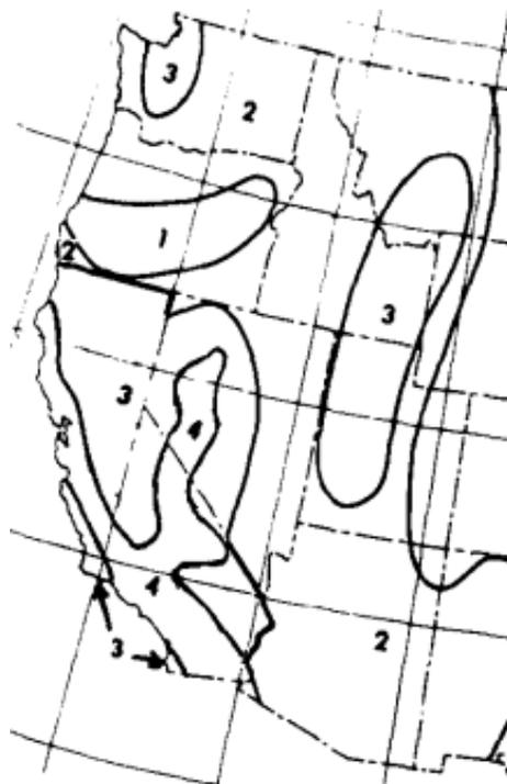
**Figure 8** 1976 UBC Seismic Zones in Washington State
