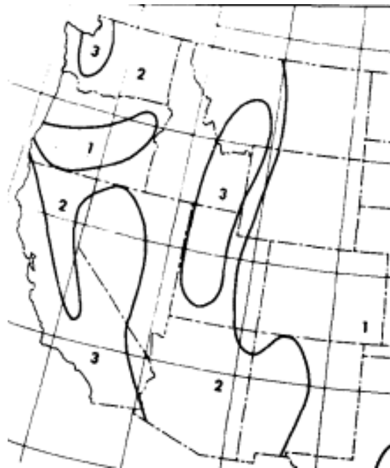
Figure 6 1970 UBC Seismic Zones in Washington State
