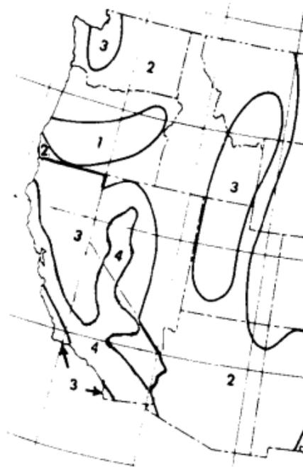
**Figure 9** 1979 UBC Seismic Zones in Washington State
