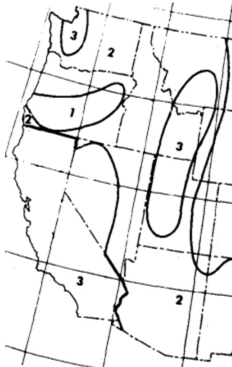
**Figure 7** 1973 UBC Seismic Zones in Washington State
