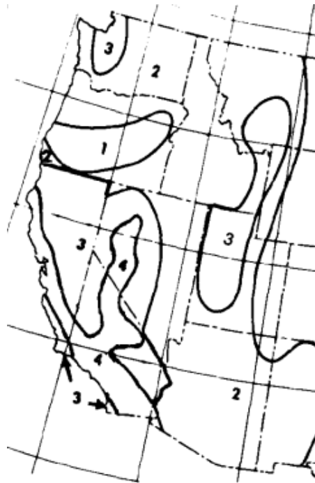
Figure 10 1982 UBC Seismic Zones in Washington State
