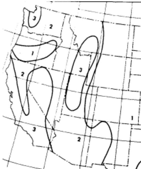
**Figure 6** 1970 UBC Seismic Zones in Washington State
