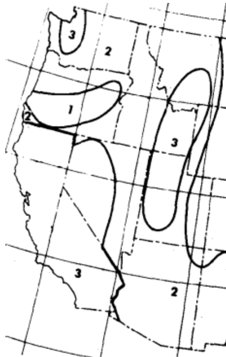
Figure 7 1973 UBC Seismic Zones in Washington State
