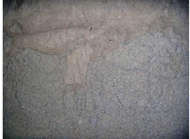
A close-up of a liquefaction feature discovered along the river banks of the lower Columbia River.
